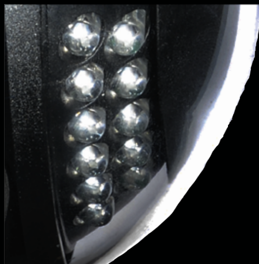
Nightvision with 22 infrared LEDs
